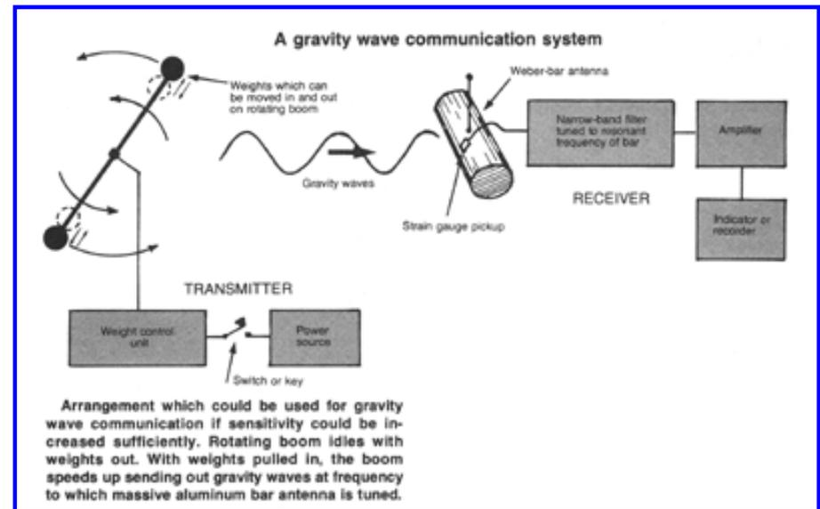
Although the message sending rate would necessarily need to be very slow and although the gravity waves might be much too weak to be practical, (like 30 or more orders of magnitude too weak) the arrangement illustrates the basic elements required for a gravity wave communication system.
