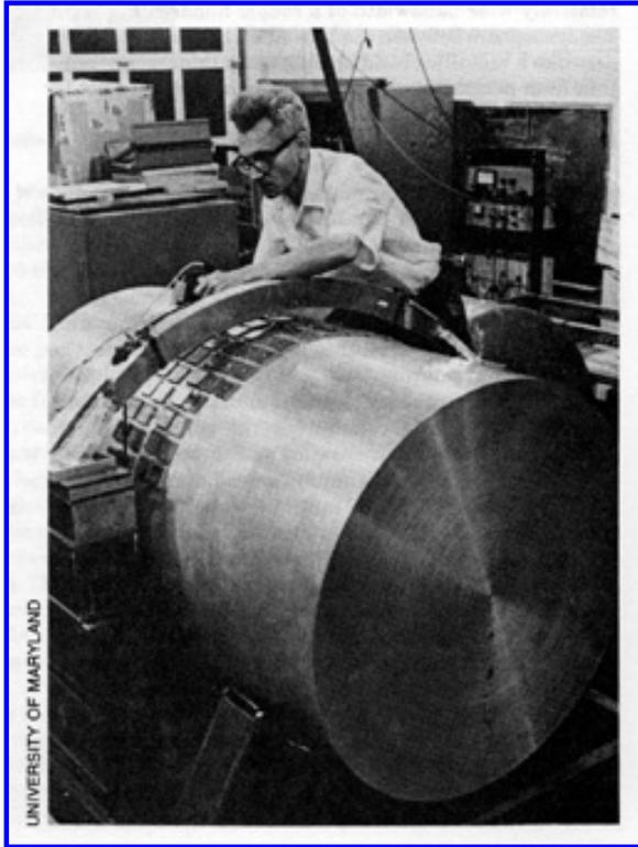
[Caption for Photo to the Left.] **Joseph Weber adjusting sensors on his big cylindrical aluminum bar often called a "Weber-bar antenna". The bar is suspended from its mid-point and during observations is enclosed in a sound-proof, shock-proof chamber from which the air is pumped out.**
